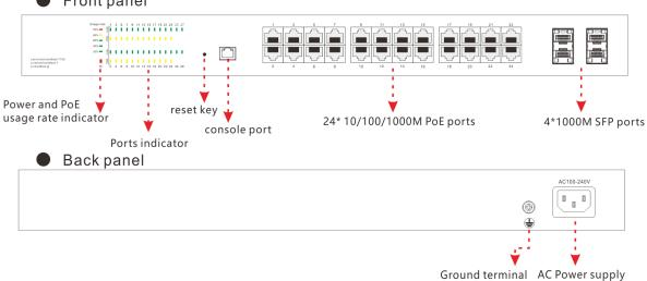
Attention 1: This product must be well grounded against lightning, please use better than 20# cable to connect the grounding terminal and ground.
